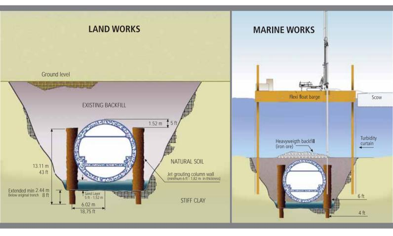
When the Estuary was deepened in the 1950s, and cover over the tunnel was reduced, heavy iron ore mixed with sand was dumped over the Posey tube to stabilize it.
