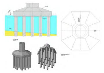
The biggest technical challenge Trevi has to face lies in the execution of those wide and long diameter piles off-shore, in the middle of the much congested and busy marine channel. Due to the large size of the piles, along with the heavy weight of their matching steel reinforcement cages, the use of huge drilling rigs, heavy machineries and equipment is mandatory. Therefore, the logistics management of the project as a whole is certainly another big challenge for Trevi.
